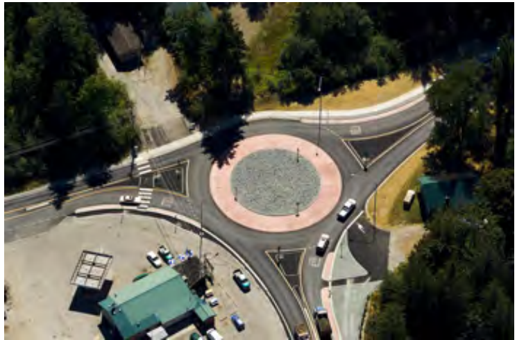
Figure 3. Single Lane Roundabout 1
